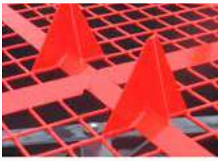
2 tear-up tips for opening the bags.
