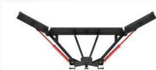
Side sections can be tilted individually hydraulically, swivel range 120°
