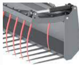
Hydraulic upper gripper with two double-acting, end-cushi- oned hydraulic cylinders
