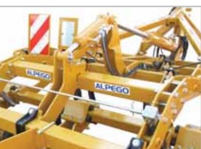
Hydraulic adjustment of the roller
